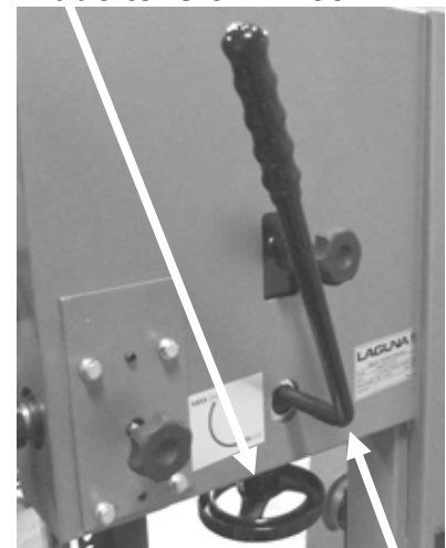
Quick action blade tension lever (activated)
