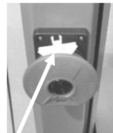
Start/stop with safety removed
